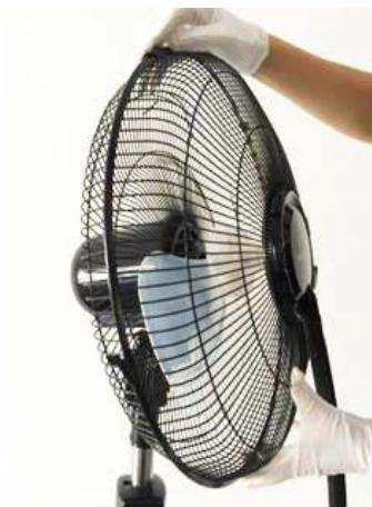
Check that the blade can rotate freely by rotating it with your hand.
