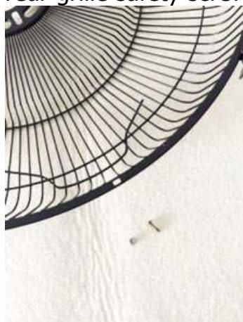
7) You must lock the bottom of the front grille with the clip at the bottom of the rear grille.
