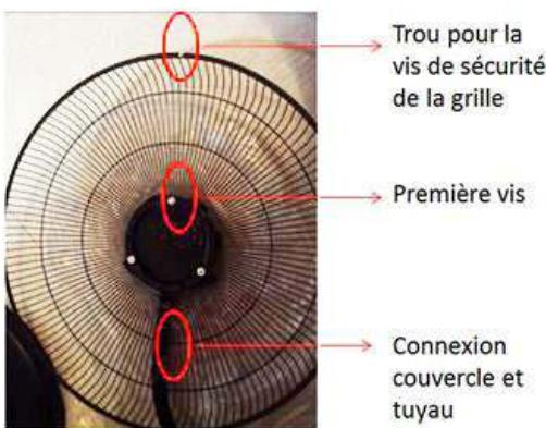
The hole for the safety screw, the first screw at the top, must be properly aligned with the pipe outlet.
